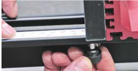
▲ Within the extrusion are sliding tapes for zeroing a setting
